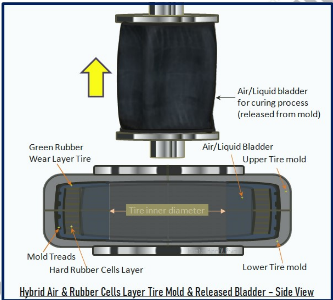
Figure-M: Hybrid Tire with Semi-Transparent Mold after Curing Process
